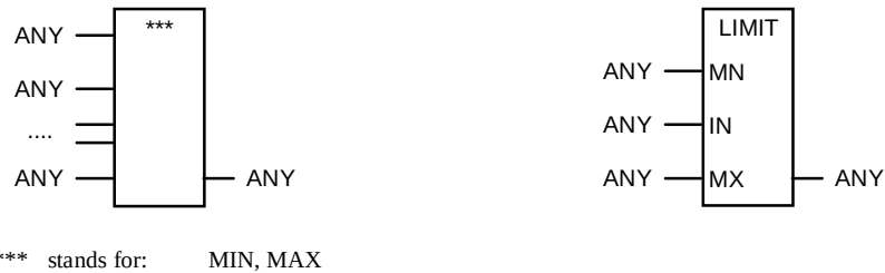
Figure A.7. Graphical declarations of the selection functions MAX, MIN and LIMIT
