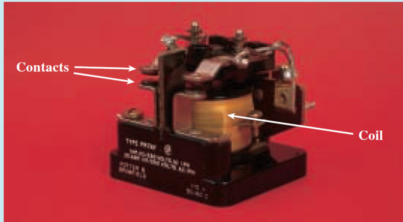
FIGURE 12-33 A typical relay.
