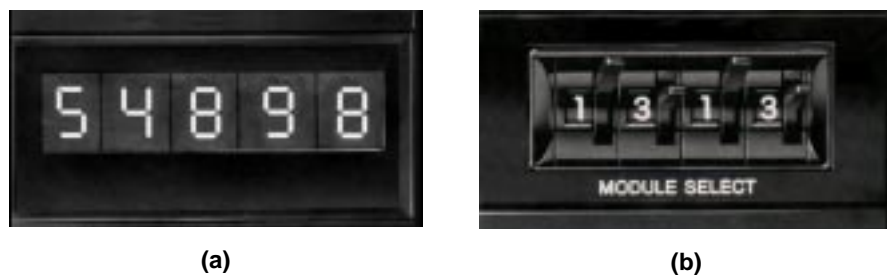
Figure 2-7. (a) A seven-segment indicator field device and (b) a thumbwheel switch.
