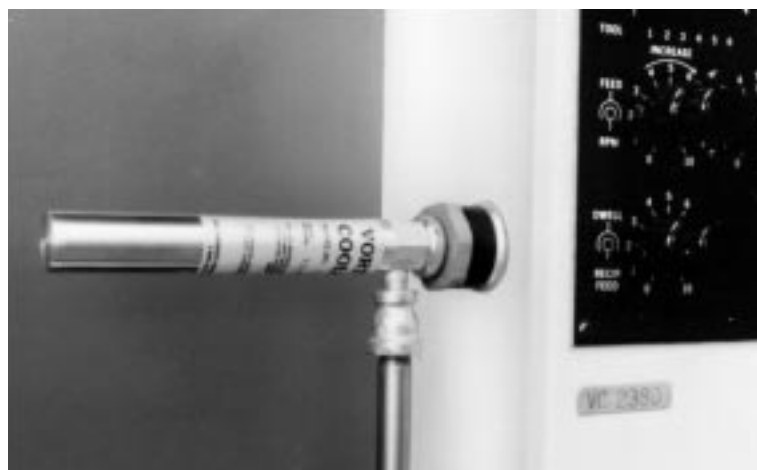
Figure 20-12. Vortex cooler used in cooling systems.
